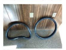
Strange things can happen to equipment in severe service. Welds joining the valve seats to their bodies were found broken and one of the seats badly deformed
