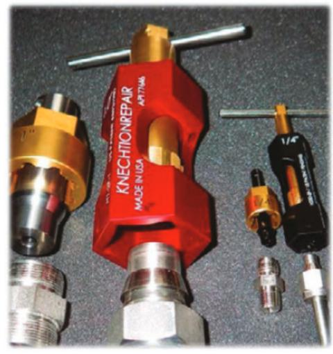
Our industrial standard 2 ferrule type repair kits are available in sizes for 1/4" through 1" tube fittings.
